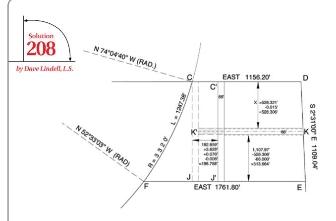
CDEF is 36 acres = 1,568,160 sq. ft., the perpendicular distance between the north and south lines is 1,107.97 and the segment area of arc CF is 48,373.60 sq. ft. Rotate 1°46'04" counterclockwise to make CD and FE "East". Drop a perpendicular from C to line FE at point J. FJ=556.903 and JE=1,204.897.
